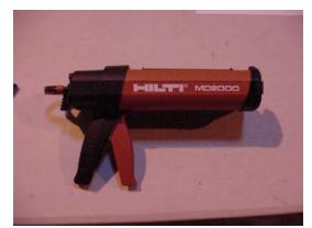
• Masonry (Hollow block, hollow clay tile, or brick with holes): Use Hilti HIT HY 20 epoxy injection adhesive, 12mm x 200mm HAS rods, and Hilti HIT-S screen tubes. Use a Hilti MD2000 Epoxy Dispenser to apply adhesive.
